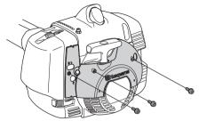
Remove the air filter and air filter cover from the machine. Fit the air filter and air filter cover supplied with the winter kit.
